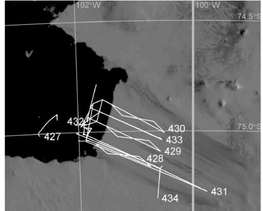
The tracks of all of the 8 Autosub3 missions carried out in the vicinity of the PIG in January 2009, superimposed on a recent MODIS satellite image. From McPhail et al. 2009.
